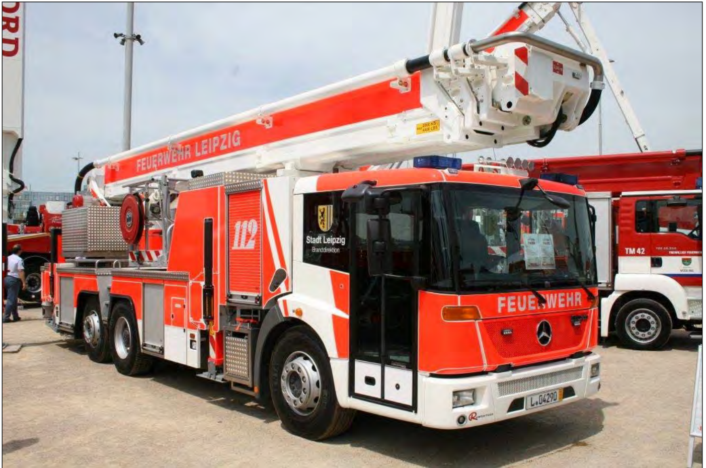
Seen at Interschutz 2012, a platform from Leipzig, Germany, this is a 46m Bronto H46 RPX on a Mercedes Econic chassis. Below is another Bronto, a TM42 RPX on a MAN chassis, from a volunteer brigade.
