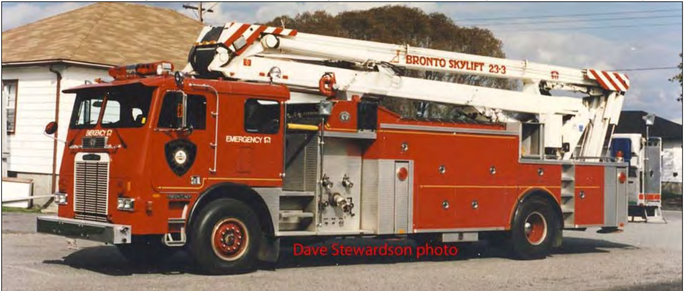
One of the early Langley built Brontos, this 1988 rig went to Sudbury. The Freightliner FLL/Anderson/Bronto product had a 1500igpm pump and a 23m tower. (Dave Stewardson photo)
