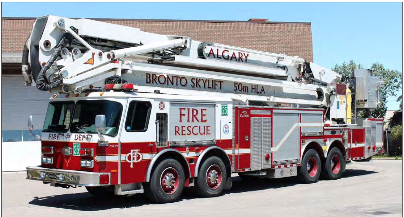
Calgary still has this 1998 E-One Hurricane/Superior/Bronto 50m HLA model, which ran as Bronto 25 when this shot was taken. It has no pump or water and is now in reserve status. (Dan Goyer photo)
