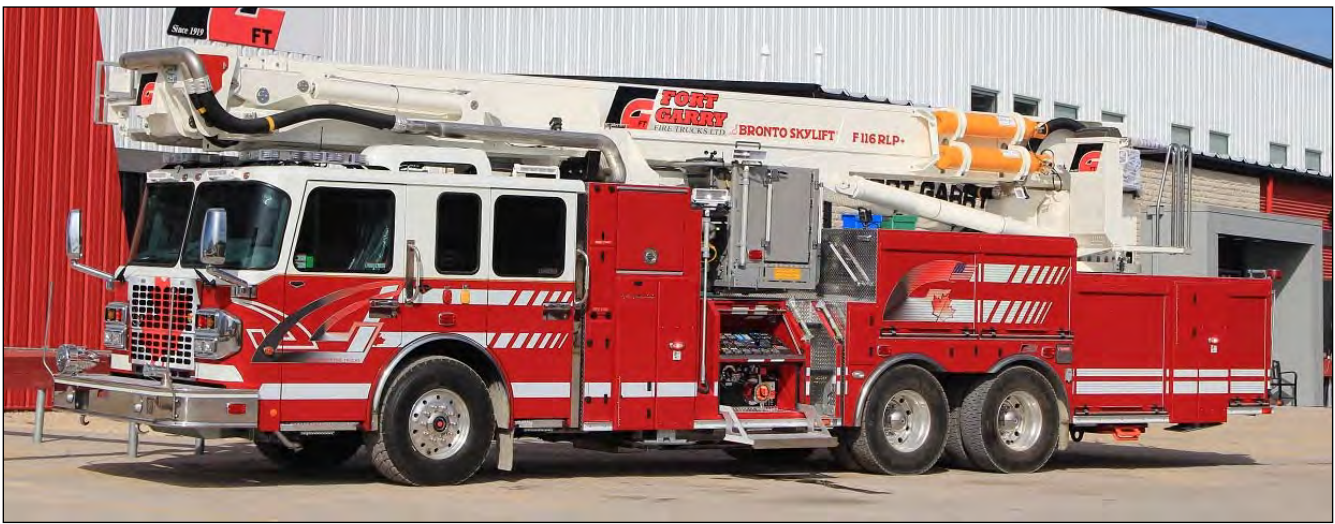
Fort Garry's original Bronto demonstrator, built last year on a Spartan Gladiator chassis. It has a 1500igpm Hale pump, 300gwt, a FoamPro 2001 foam system and a 115' tower. (Dave Stewardson photo)
