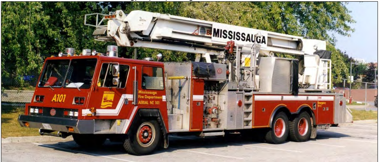
Mississauga ON A101 as a unique 1983 Pierreville Pemfab 100' aerial converted by Anderson in 1987 to a 92' Bronto. It had a 1050igpm pump and 200gwt. (Dave Stewardson photos)
