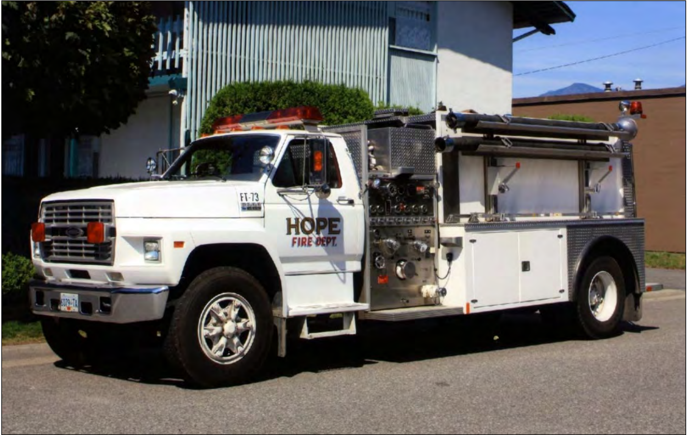
Hope, BC Tanker 1-5. 1990 Ford F800/Hub 840igpm pump/1400gwt.
