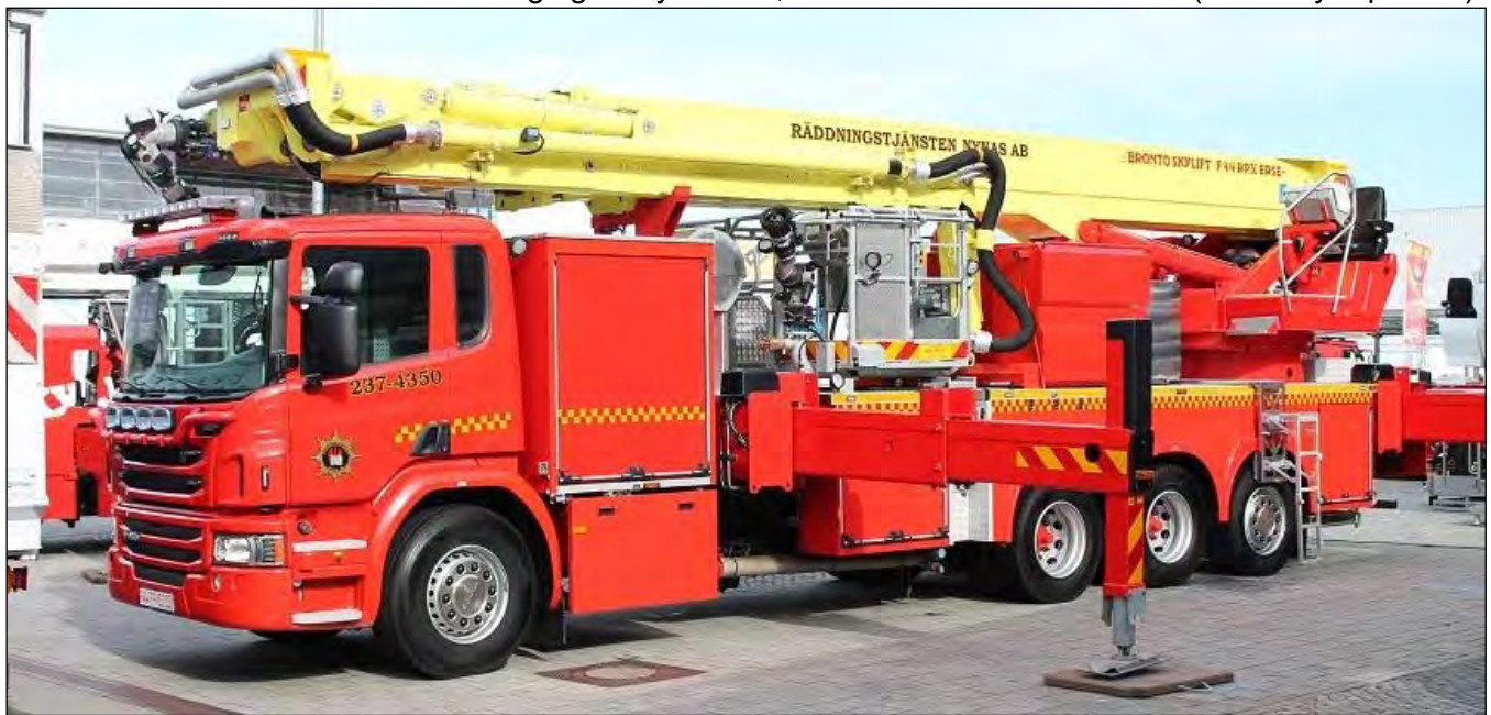
Two German Works Brigade Brontos: A 52m model on a Scania chassis with body by Zeigler, and a 44m model on a Scania P420 chassis belonging to Nynas AB, a German chemical refiner. (Dan Goyer photos)
